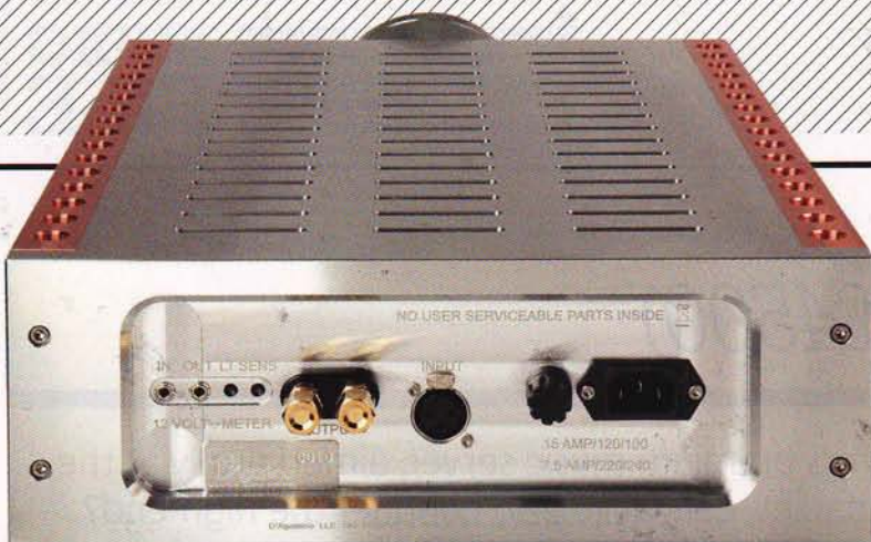
ABOVE: Each Momentum offers an XLR balanced input and single binding posts only. Note the two tiny toggle switches to operate meter sensitivity and illumination
